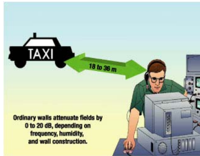
Figure 4. Distance within which a typical mobile VHF/UHF transmitter with 100-W RF power creates an RF field of 3 V/m. Actual distance depends on reflections from nearby metal objects and structures.
