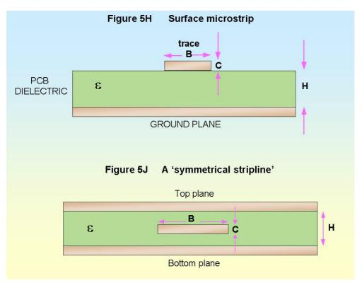
The second example is the symmetrical stripline (Figure 5J), which uses two reference planes:  $Z_o = \frac{60}{\sqrt{\varepsilon_r}} \times Ln \frac{1.9H}{0.8B+C}.$
