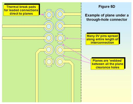
Traces, area fills, guard rings, etc. forming part of the reference on signal layers *can* be used to good effect at high frequencies – but *only* when bonded to an underlying 0V plane with at least one via hole every 5mm to 15mm (using a random allocation of spacings).
