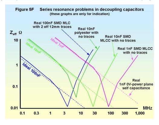
It is interesting to note that the favourite 100nF capacitor, even with no traces at all, is effectively useless above 50MHz, yet it is still often seen in circuits with clocks of 50MHz or over, where it can do nothing to help control the fundamental clock frequency, never mind its harmonics.
