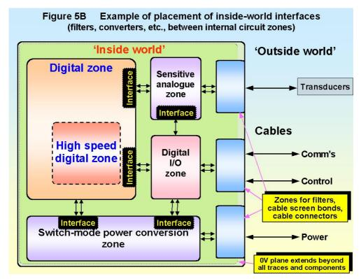
One purpose in keeping the channel component-free is to reduce crosstalk, but it also makes it easier to fit shielding over the segregated areas of circuitry, should it be needed. Where interface components like ferrite beads, common-mode chokes, or opto-isolators are placed *in* one of these channels it can help to achieve good separation between the traces associated with each circuit area, but the cut-outs they require in any PCB-mounted shield may compromise its shielding effectiveness.
