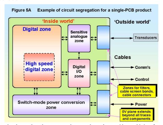
This example shows that the segregated area where the outside world interface suppression components are fitted, is along one edge of the PCB, as if it were a wall between outside and insideworlds (which it is, in a way).
