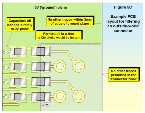
The bonds between the capacitors and the ground plane must be very short and direct, to provide the lowest possible inductance and so help the capacitors to filter out higher frequencies (see the section on decoupling, later in this Part).
