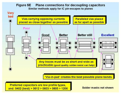
The very best method is to use 'via-in-pad'. This can be done with the standard through-hole processes by using over-sized pads and tenting a good-quality solder-resist over a number of plane vias. Via-in-pad is automatic when using Microvia (high density interconnect or HDI) PCB technology
